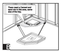
We recommend using Cement and Sand Mix or Foam underneath the shower tray during installation. This helps distribute weight evenly, reducing the risk of damage to the tray.
