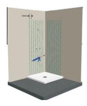
Before fitting the shower wall liner, apply a bead of silicone
