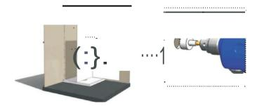
Ensure all final hole sizes have at least a 2mm clearance around tap fittings for expansion.
