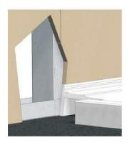
Allow the Shower Base to cure for at least 24 Hours as per the adhesive manufacturer's instructions before installing the wall sheeting. This ensures the level will not change by standing on it. sealant along the inside face of the tile bead up stand of the shower base as shown below.
